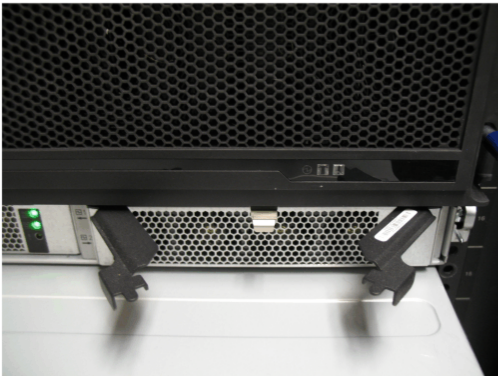
Figure 86. Releasing the power supply handles
