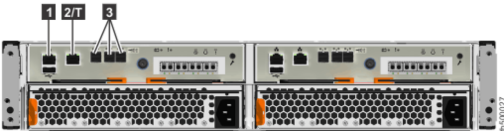
Figure 5. Data ports on the rear of the Storwize V5020 control enclosure
