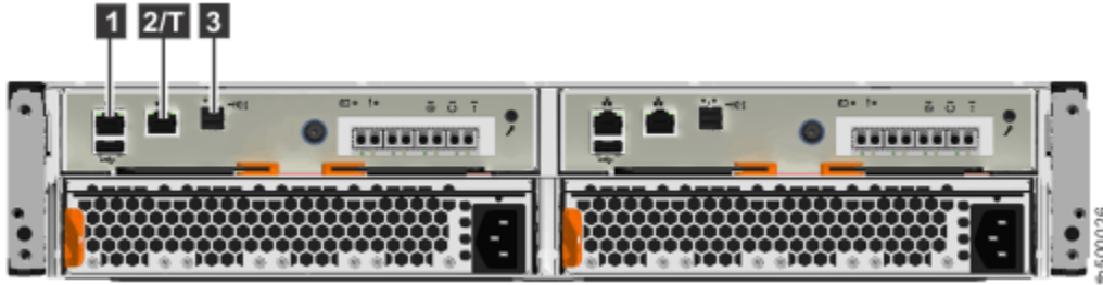
Figure 4. Data ports on the rear of the Storwize V5010 control enclosure
