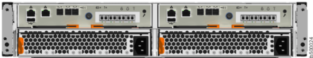
Figure 132. Example Storwize V5020 configuration with 10 Gbps iSCSI-FCoE 4-port host interface adapters
