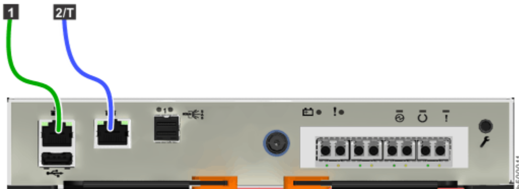
Figure 125. Connecting the Ethernet cables to a Storwize V5010 system
