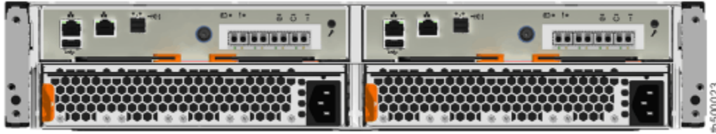
Figure 131. Example Storwize V5010 configuration with 10 Gbps iSCSI-FCoE 4-port host interface adapters
