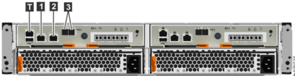
Figure 6. Data ports on the rear of the Storwize V5030 or Storwize V5030F control enclosure
