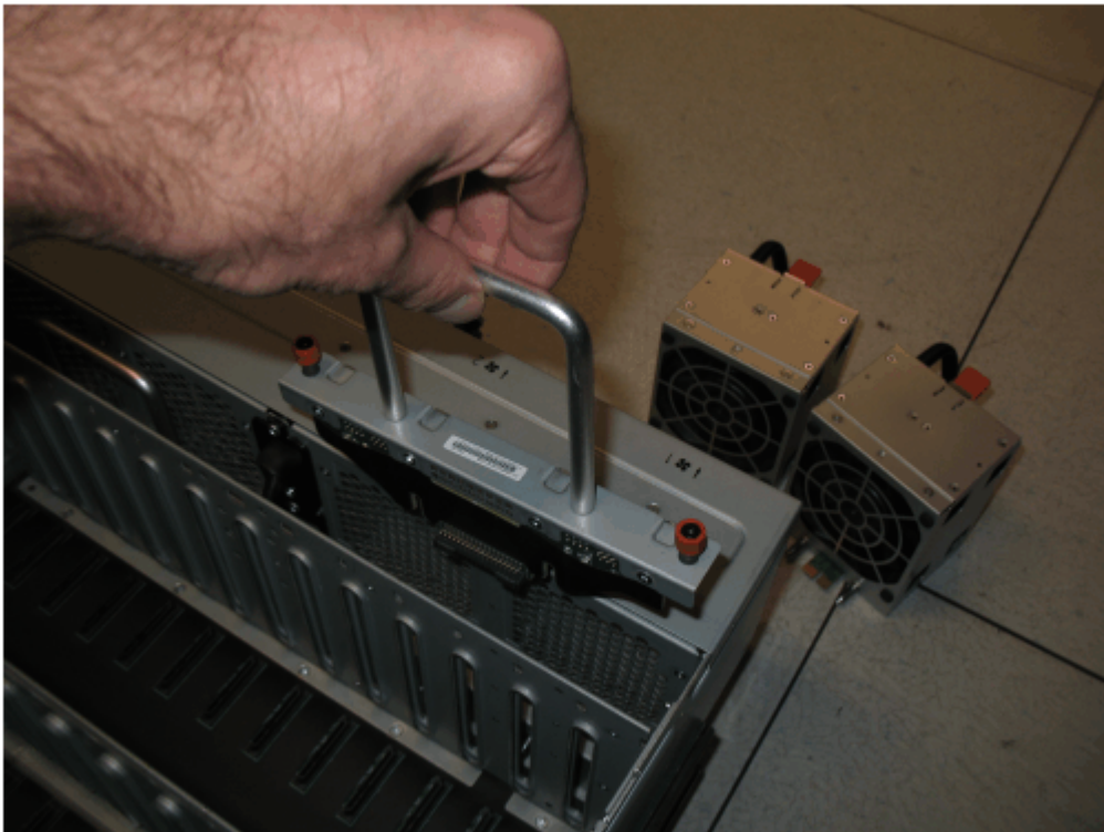
Figure 82. Insert the new FIB in the chassis
