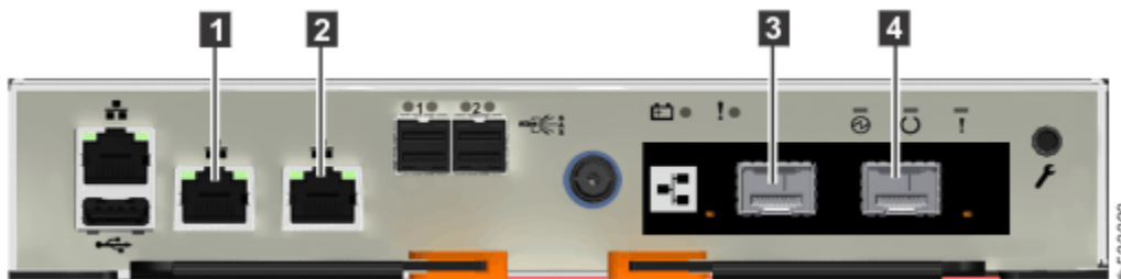
Figure 130. Example of a Storwize V5030 system with a 2-port Ethernet host interface adapter
