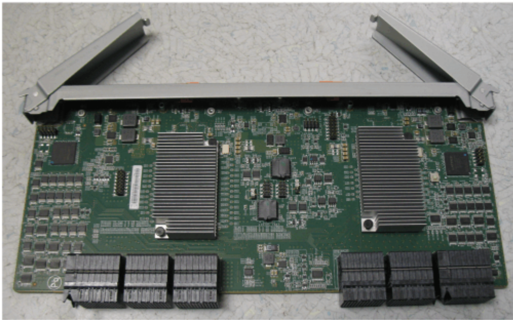
Figure 95. Secondary expander module removed from the enclosure
