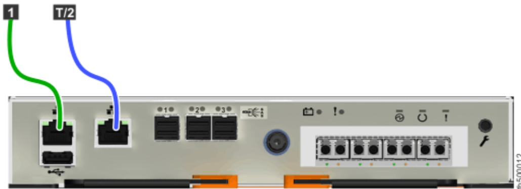
Figure 126. Connecting the Ethernet cables to a Storwize V5020 system
